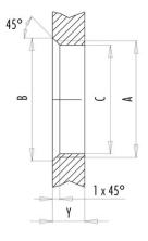
Installation direction: o-ring sits on chamfer.
